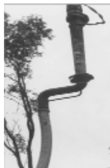
BOOM PUMP WITH DOUBLE 90° ELBOW
